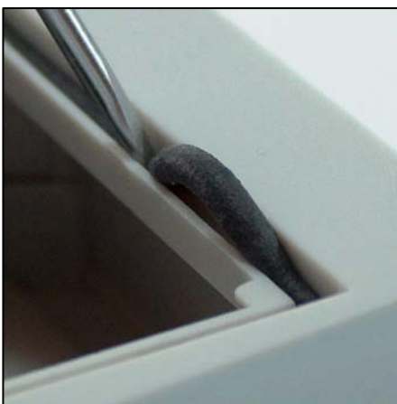
11) Fit the rest of gasket into groove
