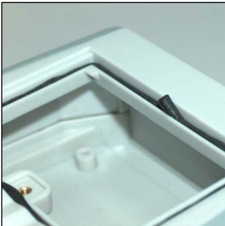
9) Fit gasket around groove, trim leaving 2-3mm loose end
